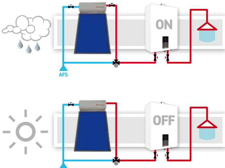
In case of insufficient solar irradiation and therefore a preheating modest water, the water heater will help with the heat needed to reach the required setpoint temperature.
