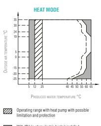
With IBH (system electric heater) installed
