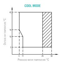
Operating range with heat pump with possible limitation and protection
