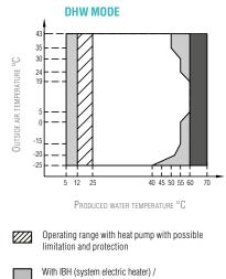
With IBH (system electric heater) / TBH (DHW electric heater) installed
