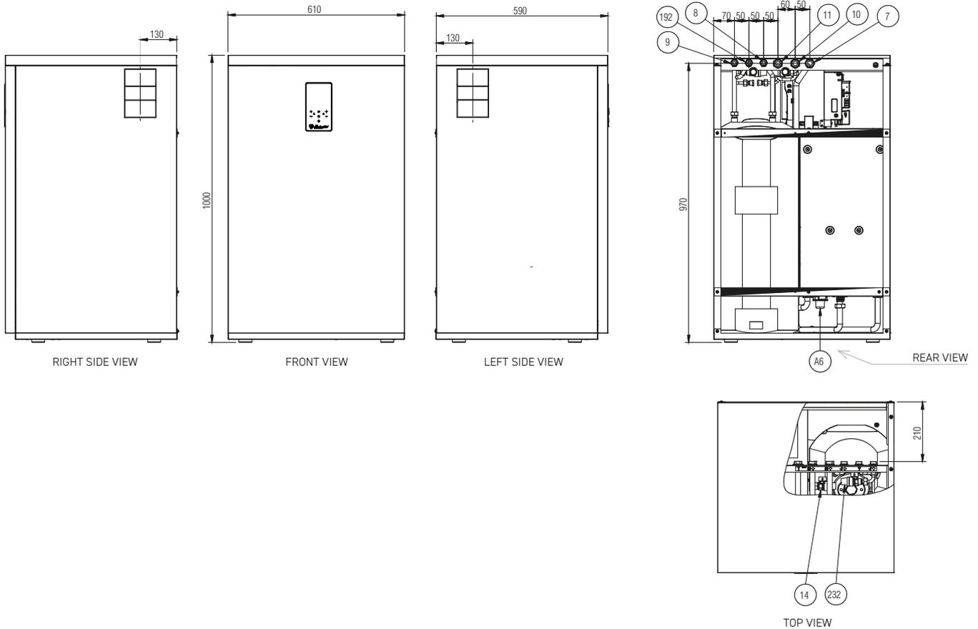
**LEGEND** 7 Gas inlet -  $\varnothing$  3/4" 8 Domestic hot water supply -  $\varnothing$  1/2" 9 Domestic hot water inlet -  $\varnothing$  1/2" 10 System supply -  $\varnothing$  3/4" 11 System return -  $\varnothing$  3/4" 14 Heating safety valve 192 Recirculation -  $\varnothing$  1/2" 232 Domestic hot water safety valve A6 Condensate drain connection
